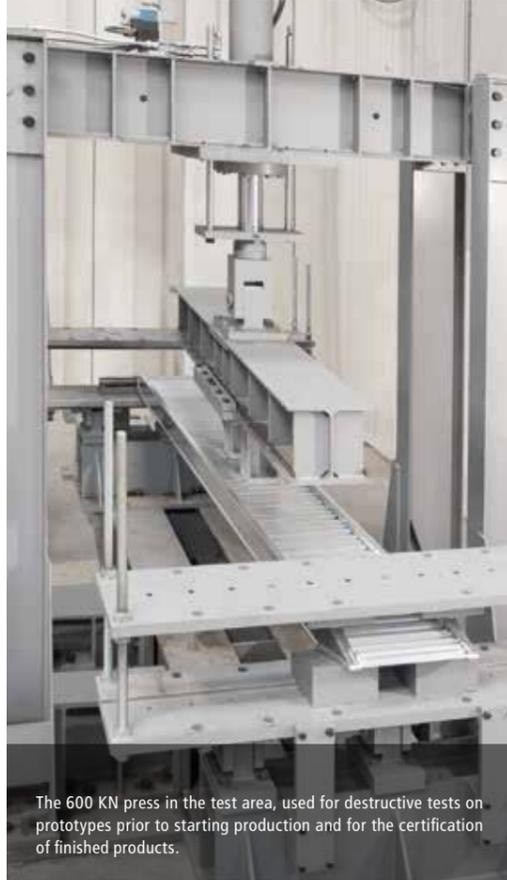
The 600 KN press in the test area, used for destructive tests on prototypes prior to starting production and for the certification of finished products.
