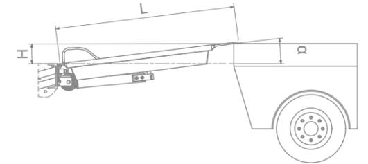
Height difference (H) refers to the height of the loading bed from the fulcrum of the bridge or tail lift.
